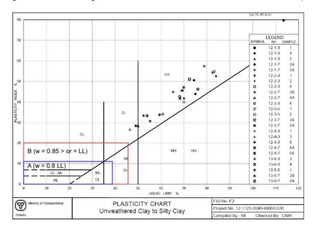
Figure 4. Type of soils which could be liquefiable showing that the soil at the landfill site are not susceptible to 'classic' liquefaction according to Seed et al. (2003). Zone A: below the blue line; Zone B: above the blue line and below the red line. In all cases, the water content has to be close to or above the liquid limit. The Leda clays tested at the Boundary Road site all fall outside regions A and B.
